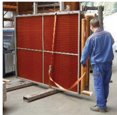
Figure 145: Securing with belt
