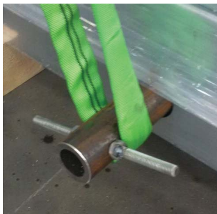
Figure 21: Securing against slipping off of the load carrying equipment
