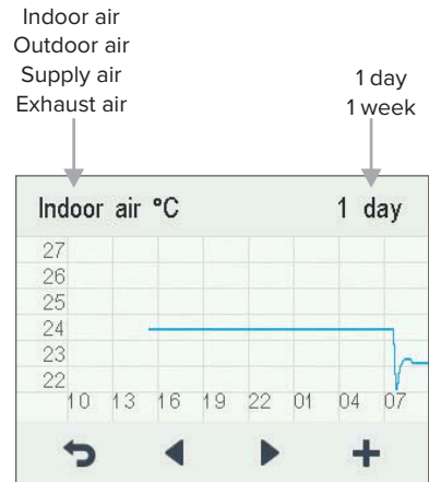
Indoor air temperature graph for the past 24 hours. The outside and supply air values are shown on a similar display. You can view the graph for a week or for a single day.
