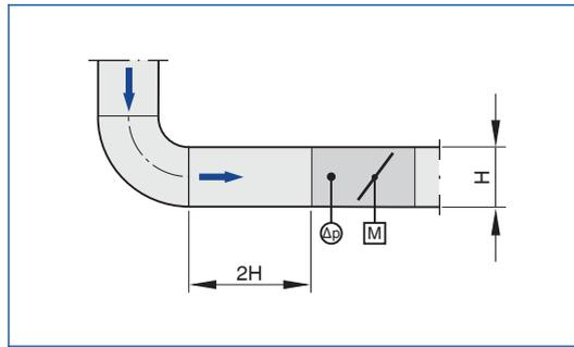
A bend – with a straight duct section of at least  $2H$  upstream of the VAV terminal unit – has only a negligible effect on the volume flow rate accuracy.
