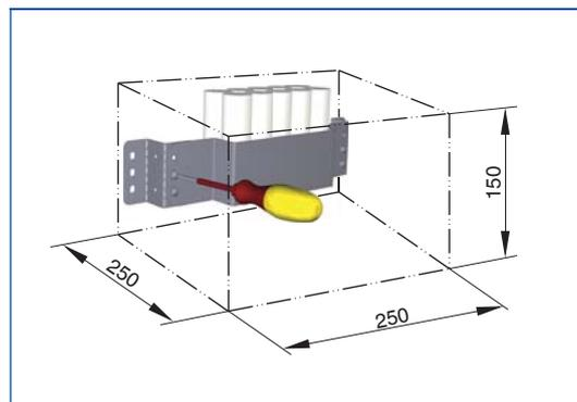
Separate space for fixing and accessing the battery pack (LABCONTROL EASYLAB accessory)
