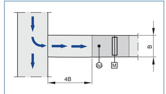
A junction causes strong turbulence. The stated volume flow rate accuracy  $\Delta\dot{V}$  can only be achieved with a straight duct section of at least  $4B$  upstream. Shorter upstream sections require a perforated plate in the branch and before the VAV terminal unit. If there is no straight upstream section at all, the control will not be stable, even with a perforated plate.
