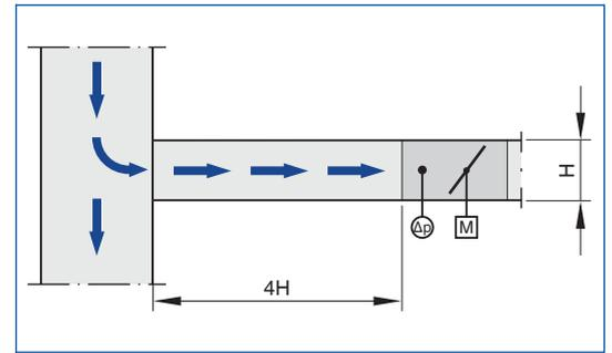
A junction causes strong turbulence. The stated volume flow rate accuracy  $\Delta\dot{V}$  can only be achieved with a straight duct section of at least  $4H$  upstream. Shorter upstream sections require a perforated plate in the branch and before the VAV terminal unit. If there is no straight upstream section at all, the control will not be stable, even with a perforated plate.
