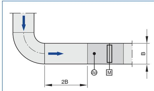
A bend – with a straight duct section of at least  $2B$  upstream of the VAV terminal unit – has only a negligible effect on the volume flow rate accuracy.
