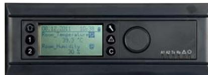
The controller has a built-in communication capability, allowing it to be integrated into a Building Management System.
