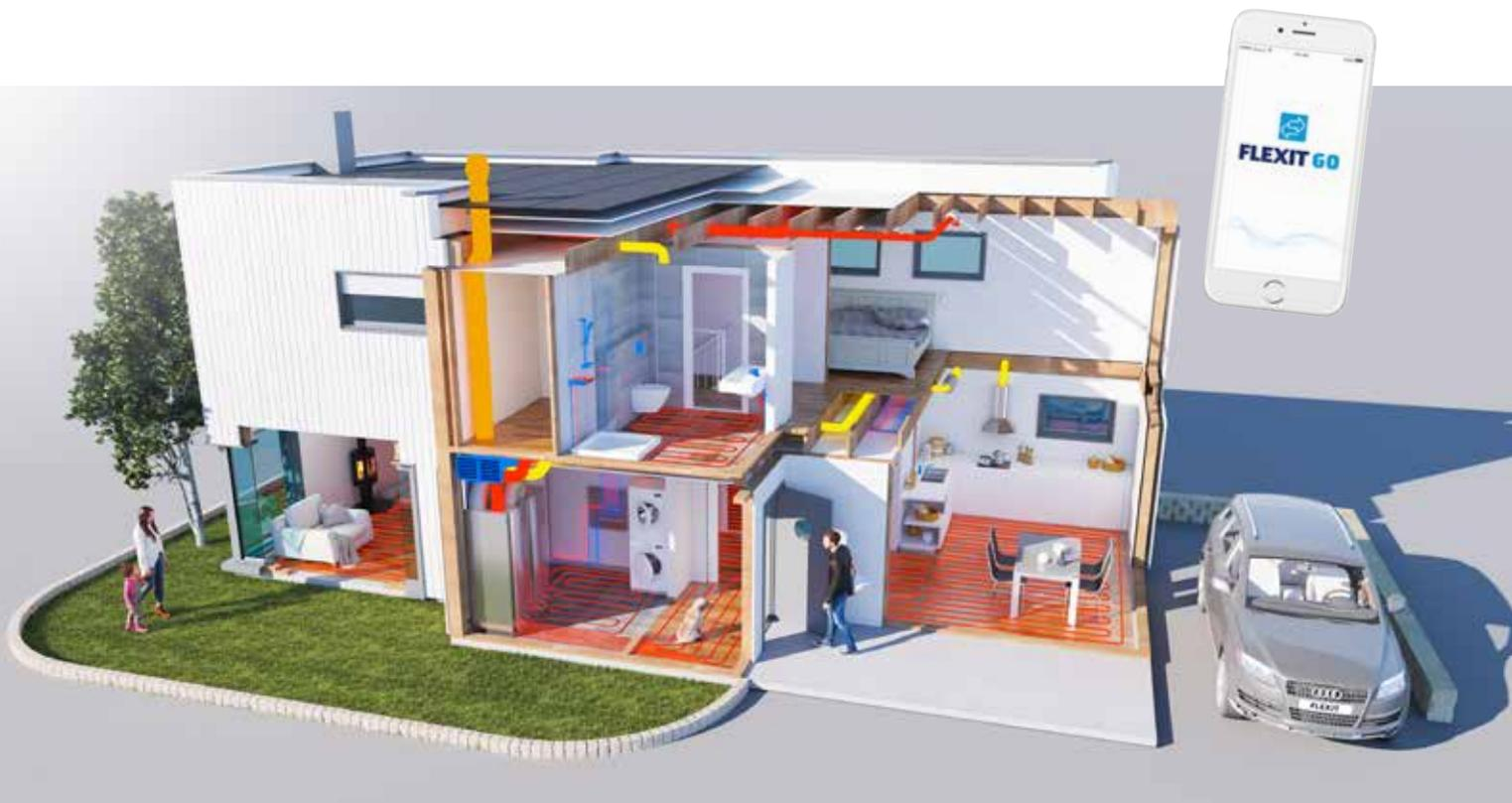
The illustration shows EcoNordic WH4 with integrated ventilation, hot water and heating installed in a plant room. The Indoor Climate Central is also available in a version without space heating (EcoNordic W4). EcoNordic is controlled with Flexit GO
